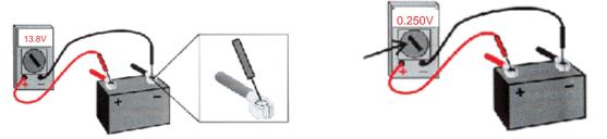
If the voltage reading is below 13.5 volts, connect the positive voltmeter lead to the output post of the alternator and the negative to the ground post of the alternator. (See diagram below.) Crank the engine and increase the RPM to a fast idle. Check the voltage reading. If the voltage reading is within range, resistance in the charging circuit is the problem. (Refer to Pg.4)
