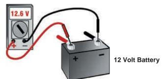
Connect the digital multimeter to the battery terminals. If your reading is 12.4 or below you must **recharge the battery before testing.**
